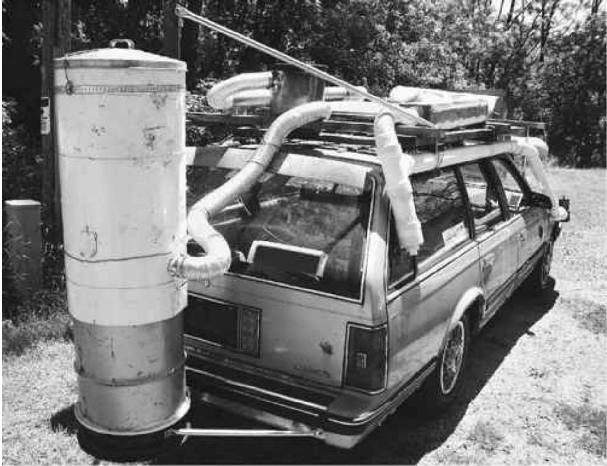
VEHICLE POWERED BY WOOD GASIFIER.
